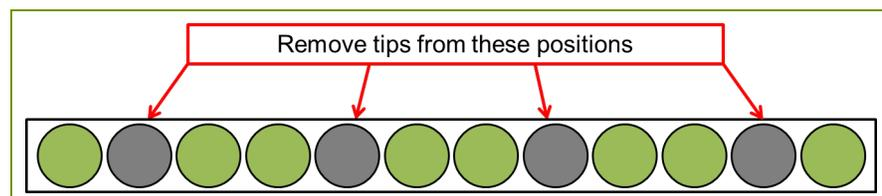
**Figure 2: Tip Loading Strategy on a 12-channel Pipettor**
